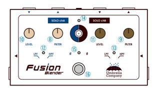
**89** Filter Knob - Adjust cutoff frequency of the filter. It becomes 20 kHz in fully clockwise position, 60 Hz in fully counter-clockwise direction.
