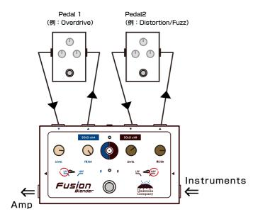
This example is FUSION(Pararell Mix/Blend) by connecting mild overdrive to channel A. Also edgy distortion (or fuzz) with on channel B. On the chB side, use FILTER to extract only the high frequebcy of the distortion sound (FILTER set on the HPF side). By setting the filter to turn to the LPF side and the FILTER knob to the clockwise side on the chA side, You can create more 3D dimentional drive sound. It is completely different from the case where two pedal.
